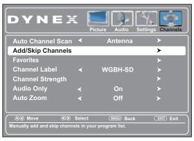
3 Press ▲ or ▼ to highlight Add/Skip Channels, then press ENTER. The channel list opens.
